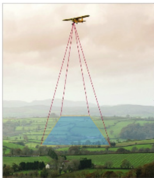
Figure 4.11: (a) Flying aircraft taking a vertical aerial photograph
