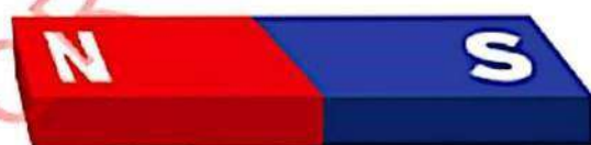
Figure 3.6: Bar magnet showing the N and S poles
