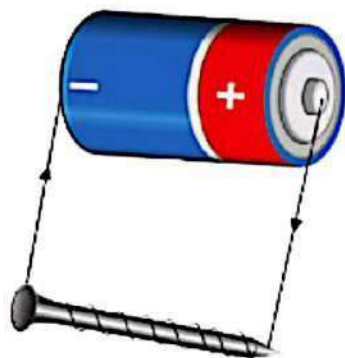
Figure 3.21: Electric method of magnetisation
