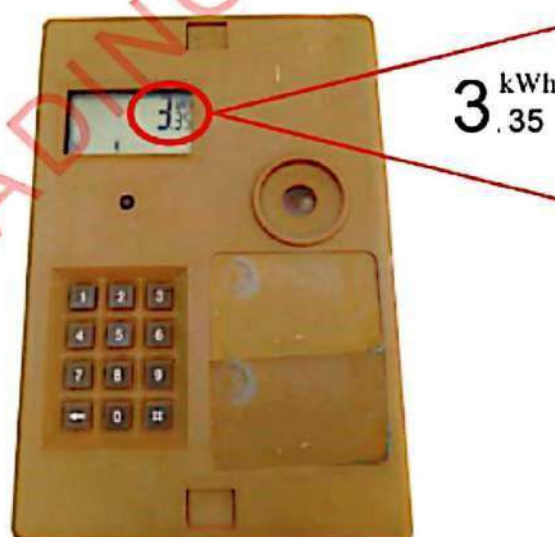
Figure 2.39: An example of a LUKU meter with 3.35 kWh (units)
