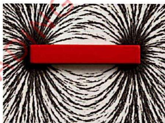
Figure 3.26: Iron filings around a bar magnet
