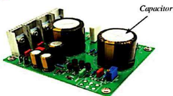
Figure 1.27: Capacitors in a radio circuit board
