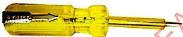
Figure 2.53: Live mains lead indicator (tester)
