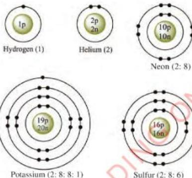
Figure 1.6: Electronic configurations of some atoms
