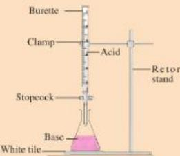
Figure 5.8: Set-up of the acid-base titration
