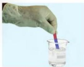
Figure 5.7: Red litmus paper immersed in an alkali solution
