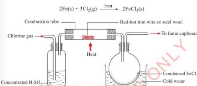
Figure 5.14: Set-up of the direct preparation of iron(III) chloride
