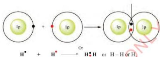
Figure 3.4: Covalent bonding in a hydrogen molecule
