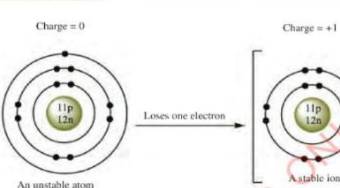
Figure 3.2: Electron arrangement in sodium atom and its ion
